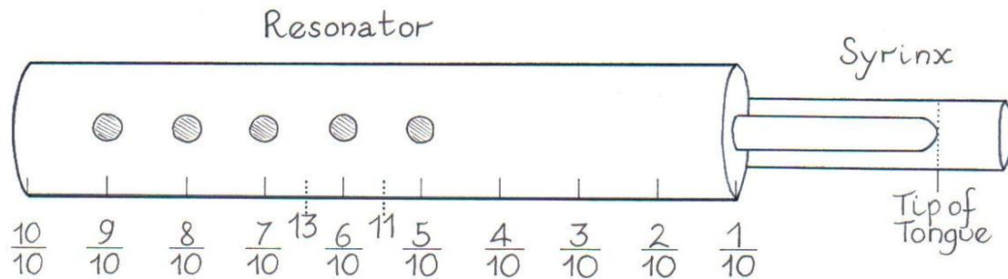
The pipe must be measured from tip of the tiny tongue to the exit in 10 equal divisions, with the mouthpiece at one increment of distance from the resonator. To get a complete octave scale a hole between 5 & 6 = 11 (perhaps on back of resonator) and between 6 & 7 (13) would have to be bored, as 7:6 and 6:5 are thirds.
