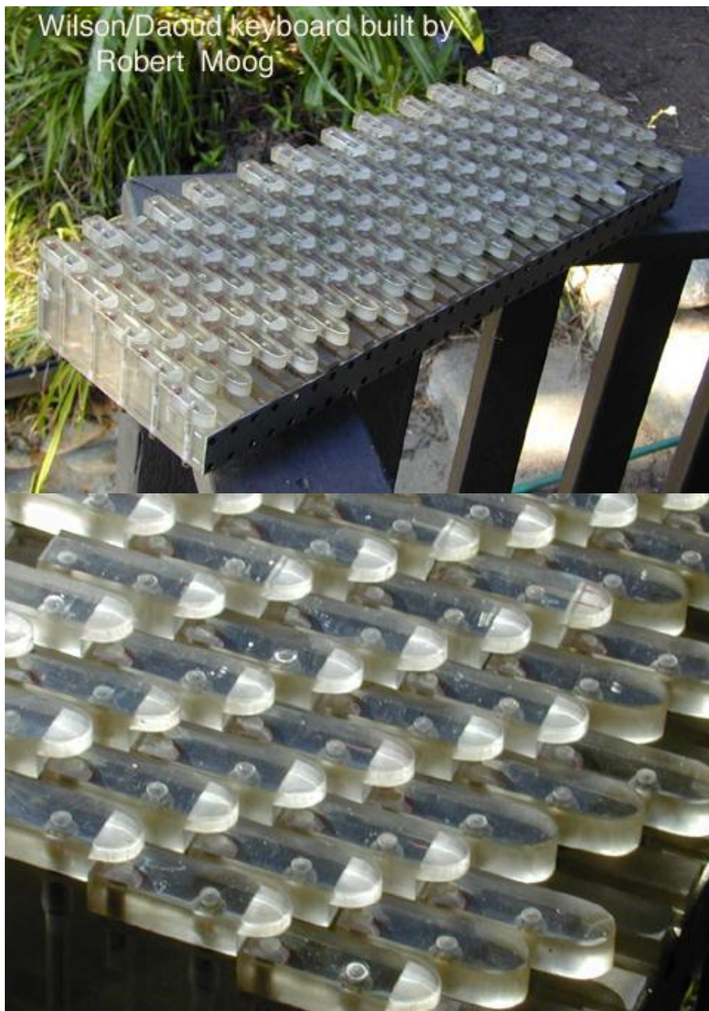
Web Figure 2.3. 22-tone generalized keyboard designed by Erv Wilson for Gary David and built by Robert Moog. Photo courtesy of Kraig Grady.
