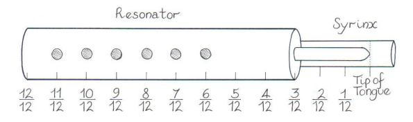
This mouthpiece has an extrusion of 3 increments of distance.
