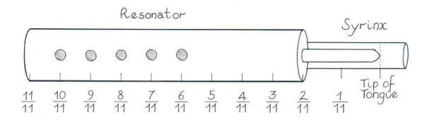
Here the mouthpiece (Syrinx) has an extrusion of 2 equal divisions.
