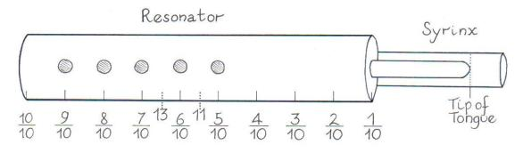
The pipe must be measured from tip of the tiny tongue to the exit in 10 equal divisions, with the mouthpiece at one increment of distance from the resonator. To get a complete octave scale a hole between 5 & 6 = 11 (perhaps on back of resonator) and between 6 & 7 (13) would have to be bored, as 7:6 and 6:5 are thirds.
